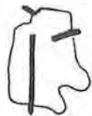
Fiber protrusion <5:1 Aspect Ratio
